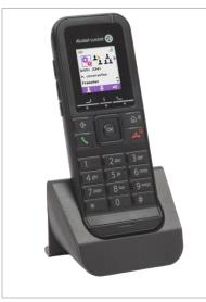
Put your phone on its support. Plug the USB cable into a 5V socket (AC/DC adaptor, computer, ...). The AC/DC adaptor is not provided with the set. Please contact your provider for a recommended AC/DC adaptator.
