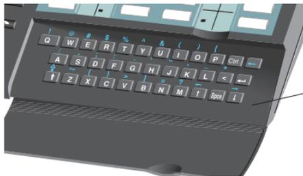
The keypad is used for text message features, the "Dial by name" feature, and for programming.
